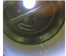
This level of aeration will register the equivalent of around 5NTU as each bubble is seen as a solid particle.
