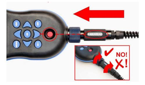
Always ensure the Aquameter<sup>®</sup> is switched off prior to connecting or disconnecting an Aquaprobe<sup>®</sup>. Align the **<Aquaread**<sup>®</sup> logo on the plug body with the red on/off switch on the Aquameter<sup>®</sup>, then press the plug into the socket and tighten the retaining collar.
