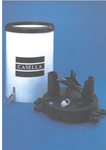
Figure 1: The non-heated tipping bucket rain gauge with the outer cover removed
