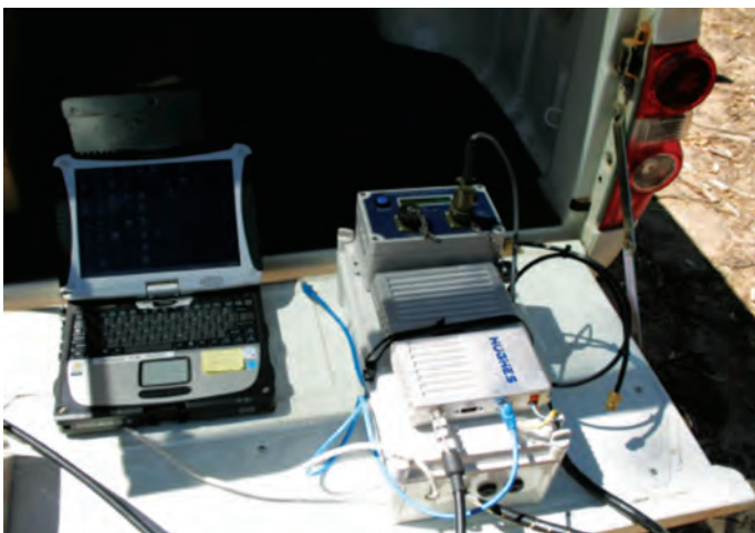
Test rig with Hughes modem, Neon terminal and SDI-12 level instrument.
