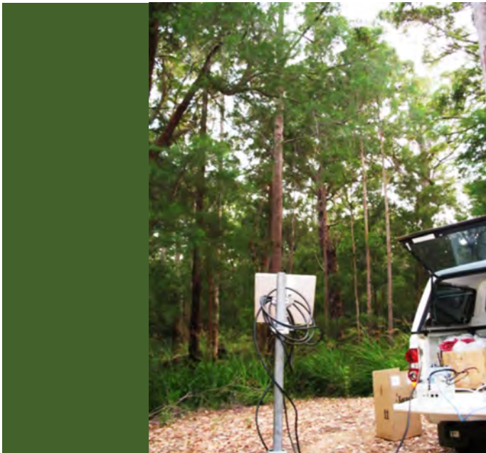
Site 5 Nornalup Forest Tall Trees (40m) with Low Understory. System connected immediately with signal strength "Narrow" and 51 and also "Region 16" and 65. Not sure why the changeover in signal strengths.
