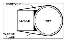
Over time temporary coupling compounds (e.g. Petroleum Gel) may gradually sag away from the sensor resulting in reduced signal strength and finally complete loss of signal. Warm temperatures, moisture and vibration will accelerate this process. Dow Corning Silicone Compound #4 as supplied with the PF D550 (and available from Micronics Limited) is recommended for semi-permanent installations.
