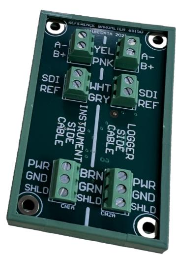
The Unidata 6515 is a barometric reference module which is used with the Starflow QSD SDI-12 instruments to correct the pressure sensor depth readings for atmospheric pressure variations.
